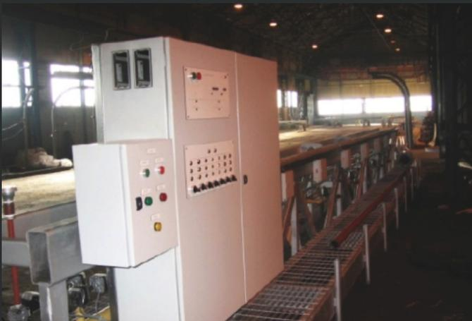
Fig. 1 Preheat rig showing control panel.
