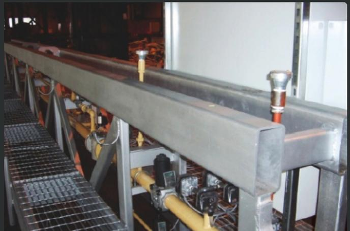
Fig. 2 Preheat rig showing gas controls.
