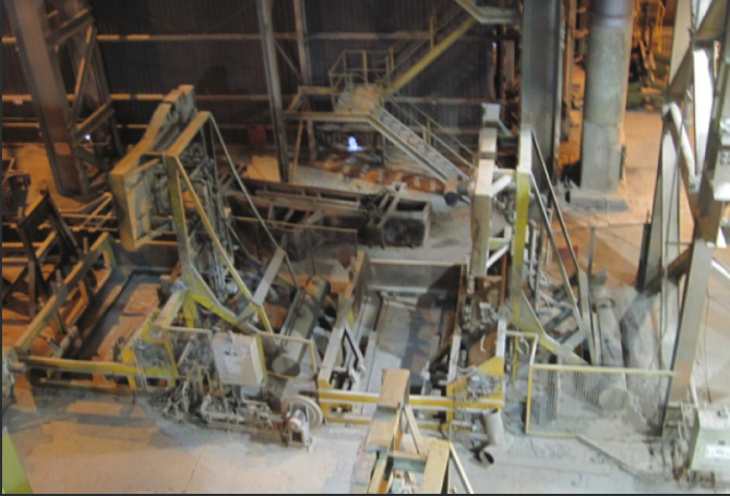
Fig. 1 Slab Dryers with "T" Outlet Burners.
