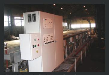
Fig. 1 Preheat rig showing control panel.
