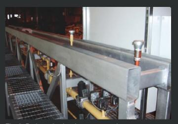
Fig. 2 Preheat rig showing gas controls.
