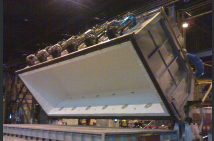
Fig. 2 Clam furnace opening (60°).
